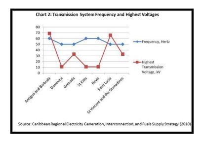
Electricity is transmitted at high voltages (120 kilovolts/kV or above) to reduce the energy losses in long-distance transmission. The information available, as at 2010, indicates that the independent ECCU member states do not transmit electricity at this optimal level (120 kV or above). Within the independent ECCU member states,
